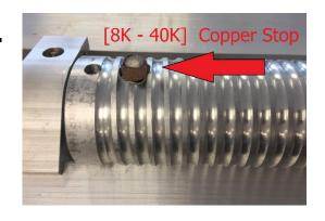
each TOP BEAM until seated firmly at cable's copper stop.
