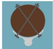
3.) Now install the (6) mounting bolts, and tighten down onto 3" x 3" square washers.
