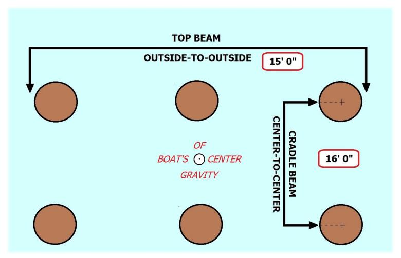
Important: Vessel's weight must be centered on the boat lift.
