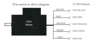
When wiring a GEM remote to a Elite Motor it is important to change the wiring in the motor to match the above diagrams. Do not assume the motor came from the supplier already wired like the above diagrams.
