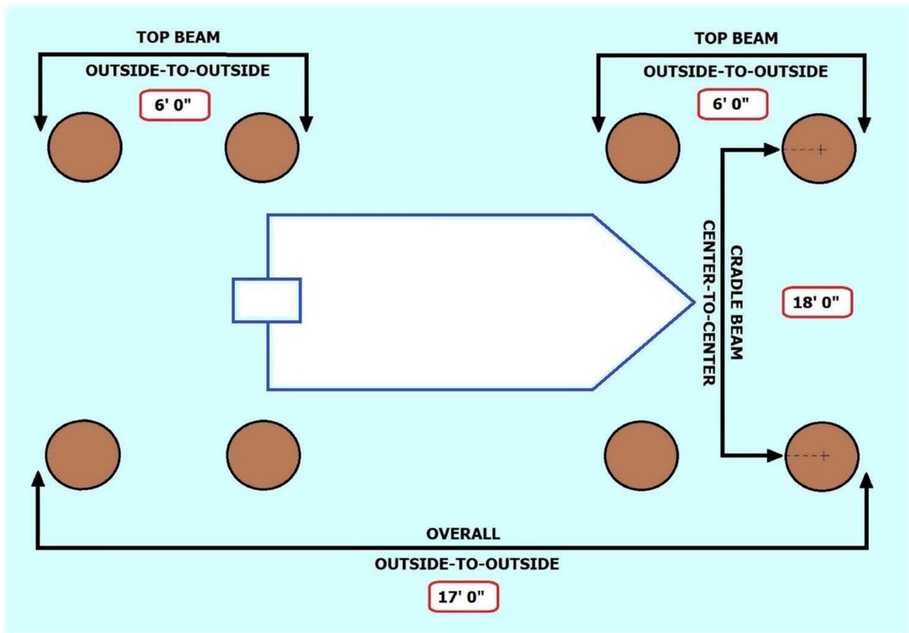
*Important: Vessel's weight must be centered on the boat lift.
